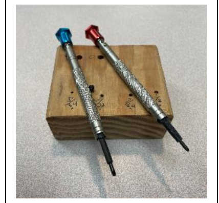
Al Johnson's Micro Mark Tools that pick up and hold small Screws for easier Assembly.
