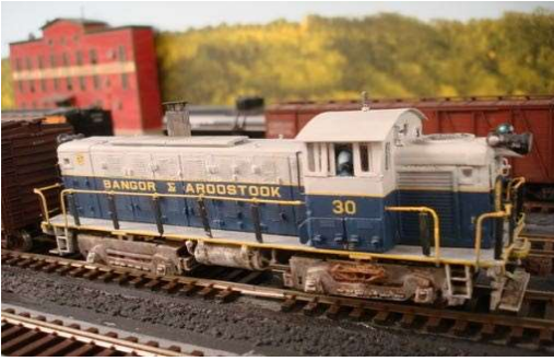
Pete Magoun scratch-built this Bangor & Aroostook Y-2 with styrene and Stanton drives.
