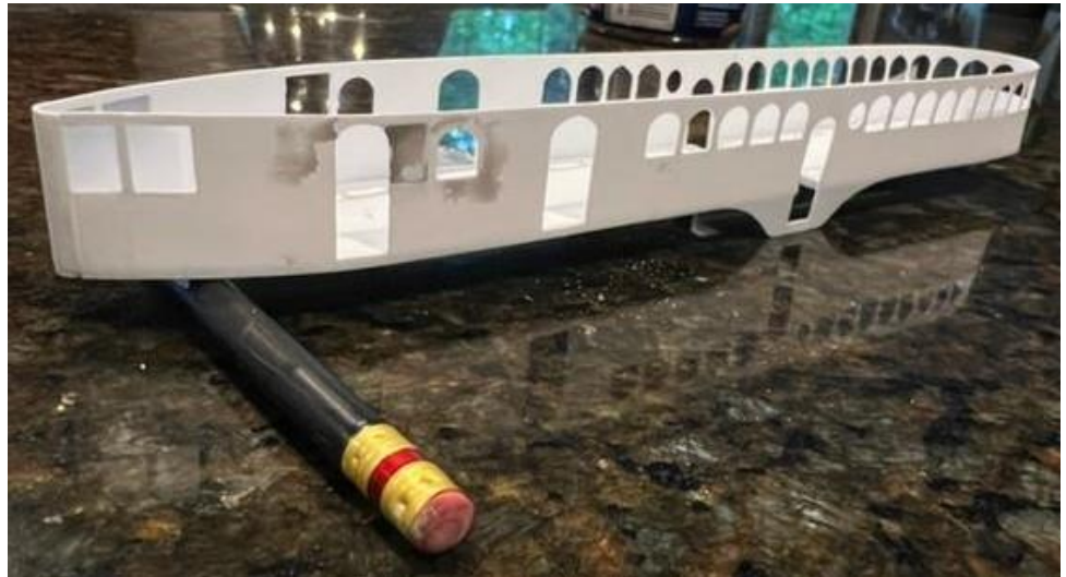
Basic structure with the car floor and car sides temporarily taped together. Gives a good idea of the basic shape.
