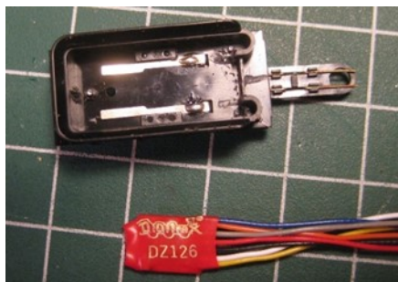
Photo 9. The tender ready for the decoder. Note solder tinned to the wiper contacts. The Digitrax DZ126 is the smallest decoder I have found, measuring .455" x .369" x .126". What also makes it attractive to me is it is transponder equipped, meaning it can be used with a Soundtraxx Surroundtraxx System in the future if I desire. Note how the red shrink tubing on the decoder hangs over the sides of the decoder board. I trimmed the red shrink tubing back as far as I could to make the form of the decoder as small as possible.
