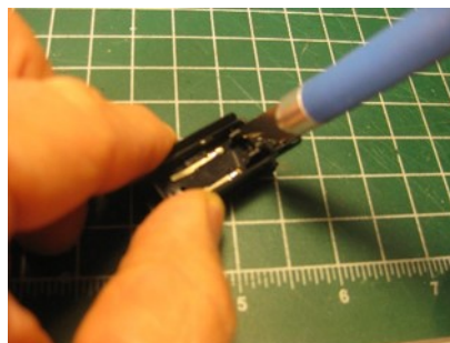
Photo 9. The tender ready for the decoder. Note solder tinned to the wiper contacts. The Digitrax DZ126 is the smallest decoder I have found, measuring .455" x .369" x .126". What also makes it attractive to me is it is transponder equipped, meaning it can be used with a Soundtraxx Surroundtraxx System in the future if I desire. Note how the red shrink tubing on the decoder hangs over the sides of the decoder board. I trimmed the red shrink tubing back as far as I could to make the form of the decoder as small as possible.
