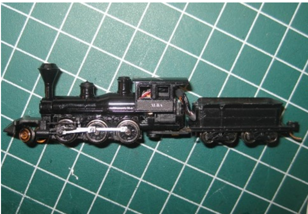
Photo 1. N scale Atlas 2-6-0 Mogul. Each square on my pad is ½". The full length of engine and tender is about 4".
